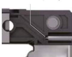
Sealed lubricant passage
