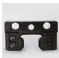
End seal in good condition
